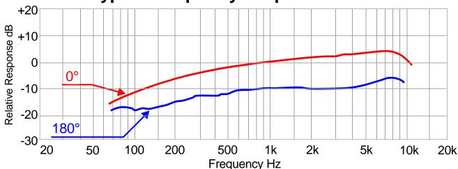
Sensitivity: -70dB ±4dB (0dB=1V/uBAR@1kHz)
